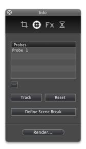
14. You can see the probe tracking progress in the control panel of the movie window. The pink line shows which part of the movie still has to be analyzed.
